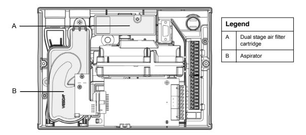
Figure 28 - Maintenance - replaceable items
