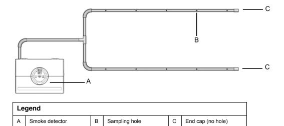
Figure 19 - Open hole, branched pipe
