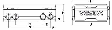
Figure 1 - Dimensions of the detector
