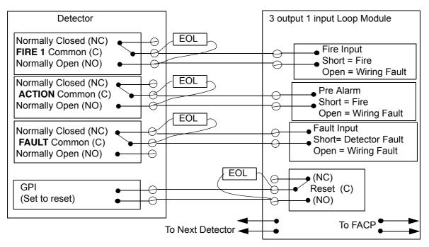
Figure 15 - Addressable Loop Module with EOL
