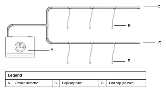
Figure 20 - Capillary pipes, branched pipe
