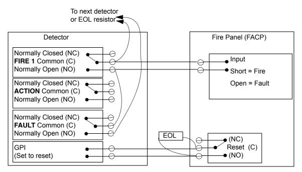
Figure 14 - Typical wiring to a fire panel with EOL
