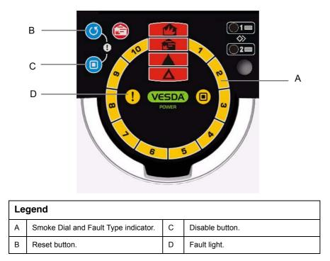
Figure 27 - Smoke level and fault condition display
