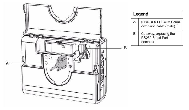
Figure 16 - 9 Pin connector and RS232 serial port
