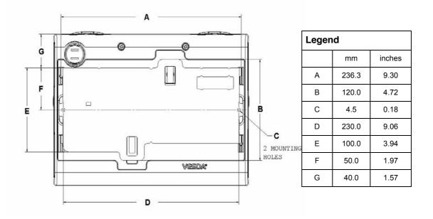
Figure 2 - Dimensions of detector with mounting bracket
