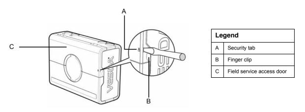
Figure 25 - Field Service Access Door security tab and clip
