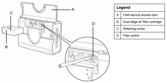
Figure 29 - Filter replacement
